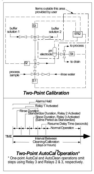
Figure 15-13 Two-Point AutoCal Operation
